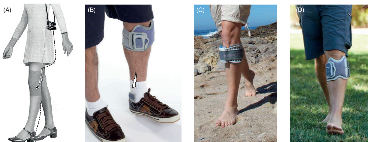
Figure 2 Four surface foot-drop stimulators that activate the common peroneal nerve to lift the foot in the swing phase of the locomotor step cycle. (A) The Functional Electrical Peroneal Orthosis (FEPO), commercialized in Europe in the 1970s. (B) The Innovative Neurotronics Walkaide. (C) The Bioness L300. (D) The Bioness L300Go. The FEPO and L300 had underheel switches wirelessly linked to an EPG in a cuff attached below the knee. When the underheel force dropped at the onset of the swing phase, a signal from the switch assembly triggered the EPG to stimulate the nerve via electrodes in the cuff. The Walkaide and Bioness L300Go have a tilt sensor built into the cuff, which is used to trigger stimulation, replacing the underheel switch and allowing users to walk barefoot.
